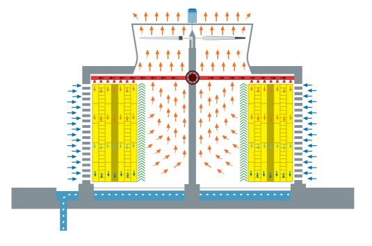
The Kelvion crossflow cooling tower operates quietly and economically and has a high cooling capacity. The modular system can be easily adjusted to suit cooling requirements and the space available. The cooling towers provide an optimal performance and problem-free operation. The considerable savings in water usage (95%+), and the exceptionally low noise level make the economical crossflow cooling towers the best choice for both people and the environment.
